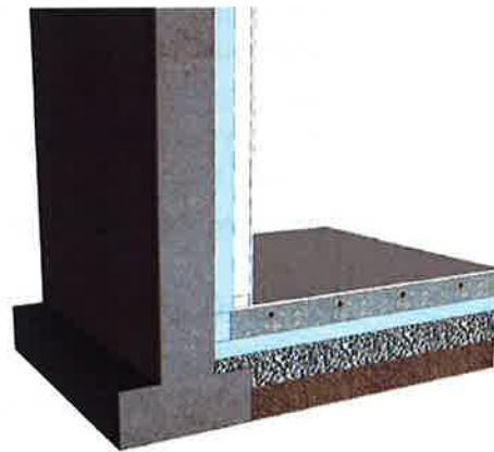
Interior wall insulation and insulation under all heated slab areas.
