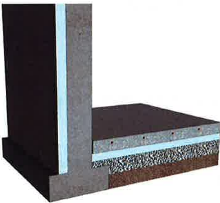
Exterior insulation to the footing and insulation under all heated slab areas.
