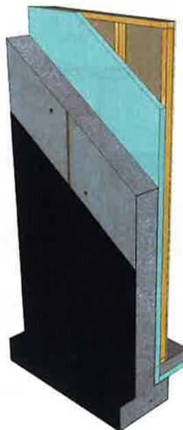
Basement Wall with Interior Insulation
