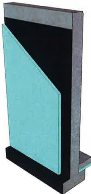
Basement Wall with Exterior Insulation
