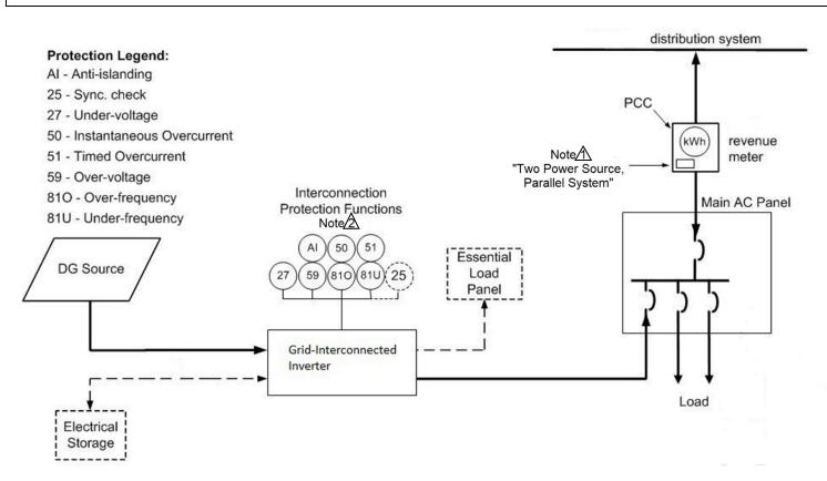
Figure 1 – Single Line Diagram of Typical Inverter Based Generator (Source: Adapted from CAN/CSA-C22.3 No. 257-06 B-1)
