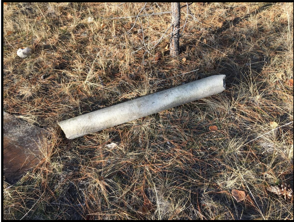
Photo 9: View of an asbestos-containing pipe observed in the southeast portion of the site. Another piece of ACM pipe was also observed within close proximity.
