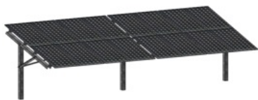
Above, a typical PV support structure with penetrating foundations
