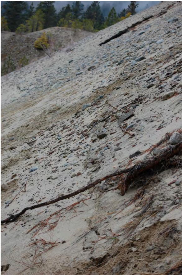
Photograph 3882 (left): Looking southwest along mid slope at recent tension crack (partially obscured by ravelled material) across sand and gravel face overlooking lower slide bench. Lack of grass, shrubs or small tree cover is indicative of ongoing ravelling from continuing creep movements.
