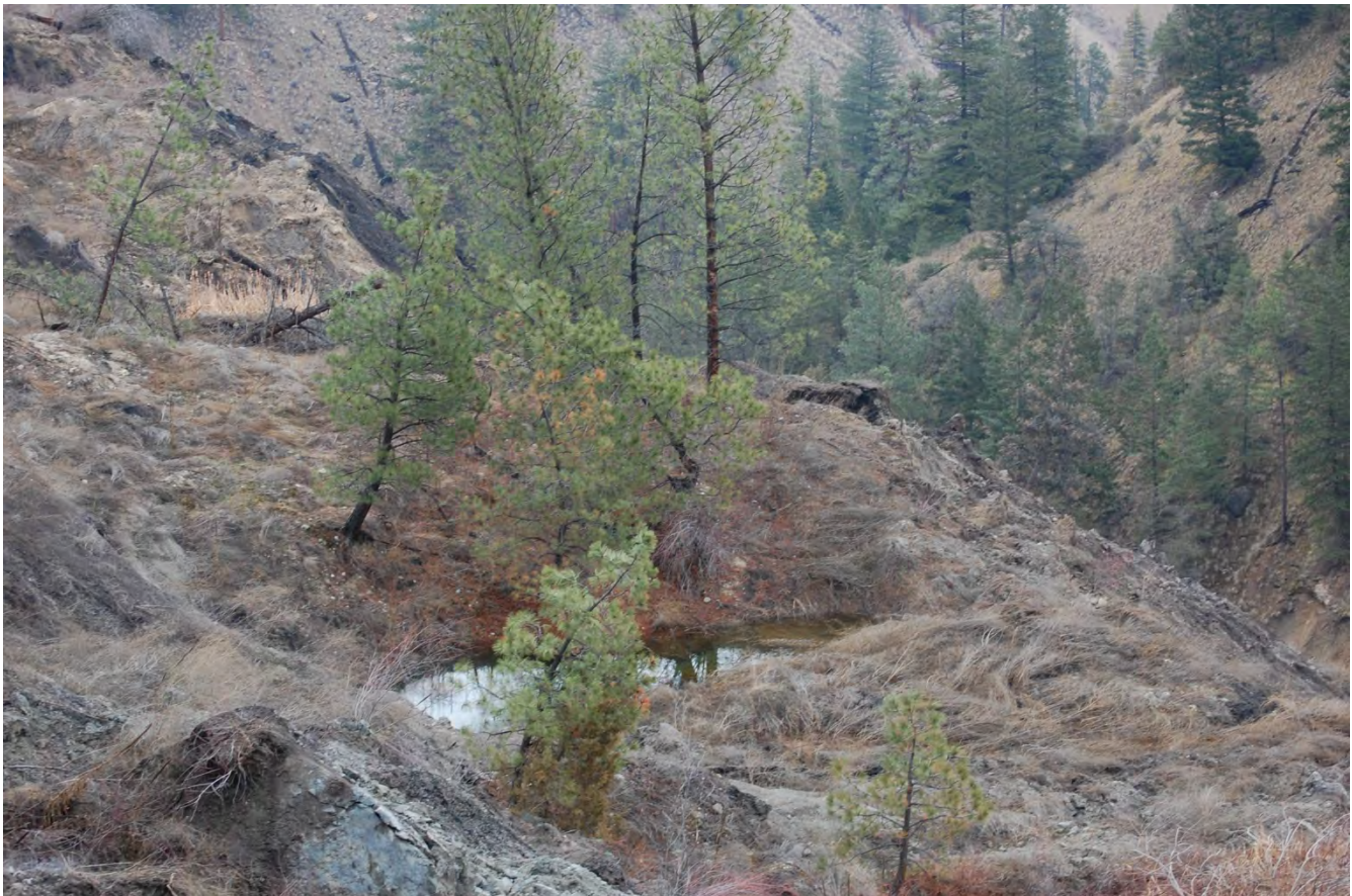
Photograph 3991: Looking southwest at large area of ponded groundwater seepage near middle of lower slide bench.
