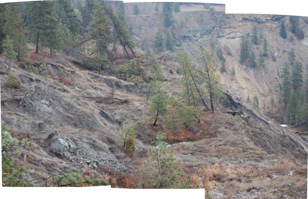
Stitched photographs 3963-3965 (below): Looking east-northeast across lower slide bench showing backward lean and rotation of mature trees by about 25 to 35 degrees from vertical. Area of numerous fresh scarp sloughs with groundwater seepage.
