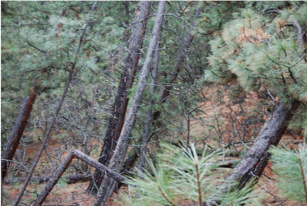
Photograph 3998: Looking west-northwest along crest of lower slide bench at rotational block failure where trees are leaning backwards into the slope, especially within graben areas. This area is located just upslope at the top left corner on the stitched photographs 3963-3965.
