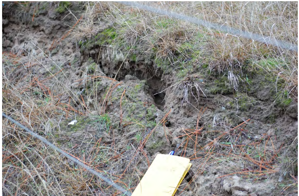
Photograph 3837: Looking southwest at fresh tension crack along slide head scarp where horizontal and vertical displacements of 10 to 15 cm exist within natural sand deposits.
