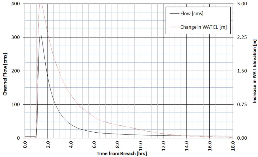
**Figure B.6 - Output for Station 12+076 - 2.5 Hour Dam Breach Duration**
