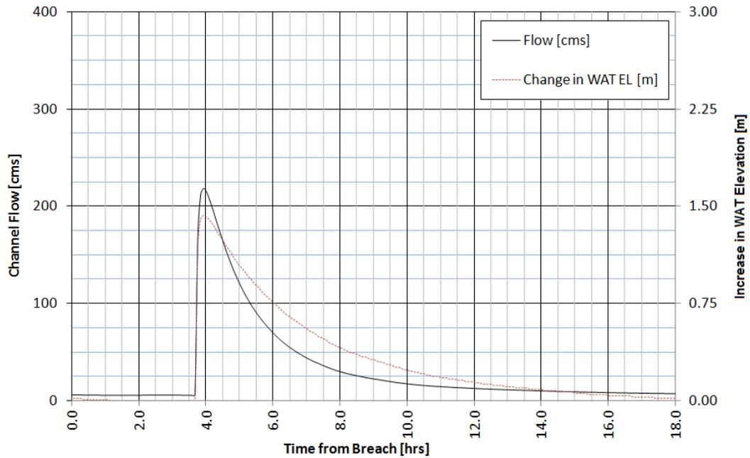
**Figure B.13 - Output for Station 2+987 - 1.0 Hour Dam Breach Duration**
