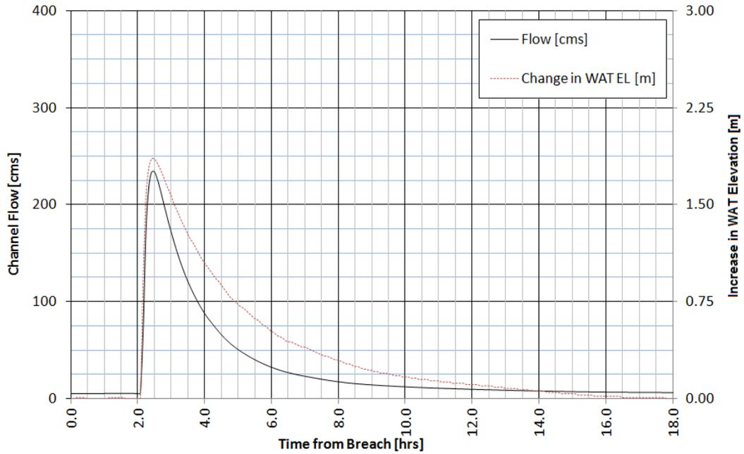
**Figure B.10 - Output for Station 6+026 - 2.5 Hour Dam Breach Duration
