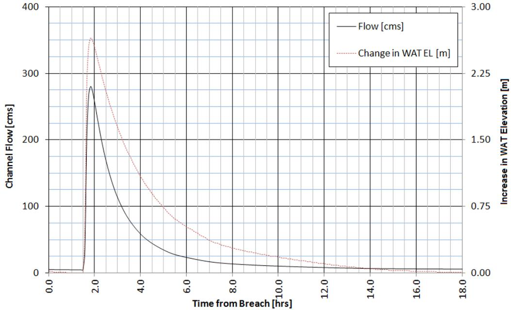
**Figure B.8 - Output for Station 8+976 - 2.5 Hour Dam Breach Duration**
