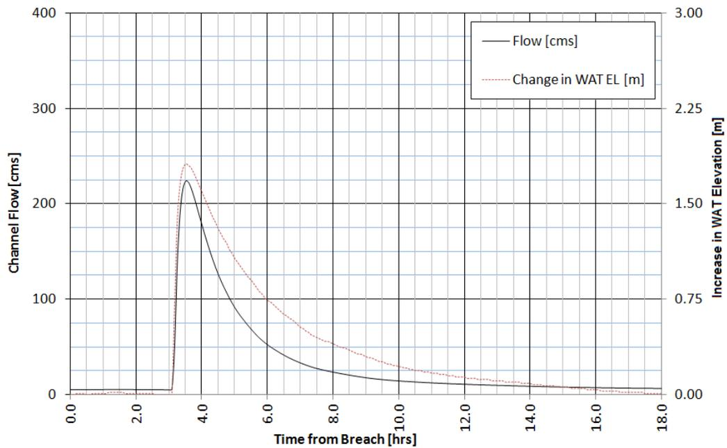
**Figure B.11 - Output for Station 4+226 - 1.0 Hour Dam Breach Duration**
