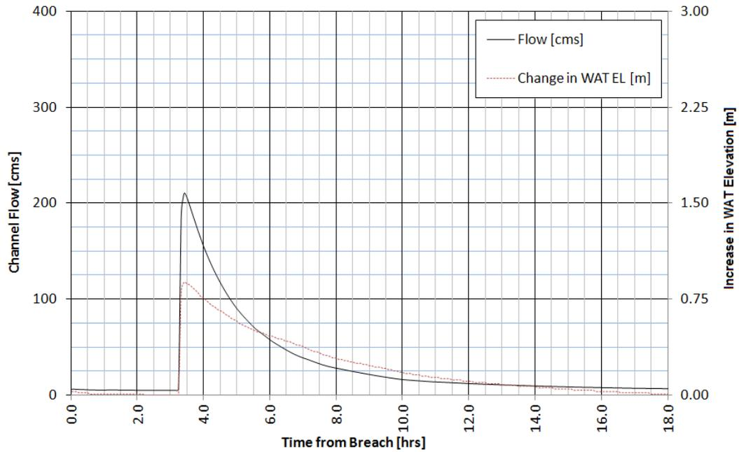
**Figure B.16 - Output for Station 2+431 - 2.5 Hour Dam Breach Duration
