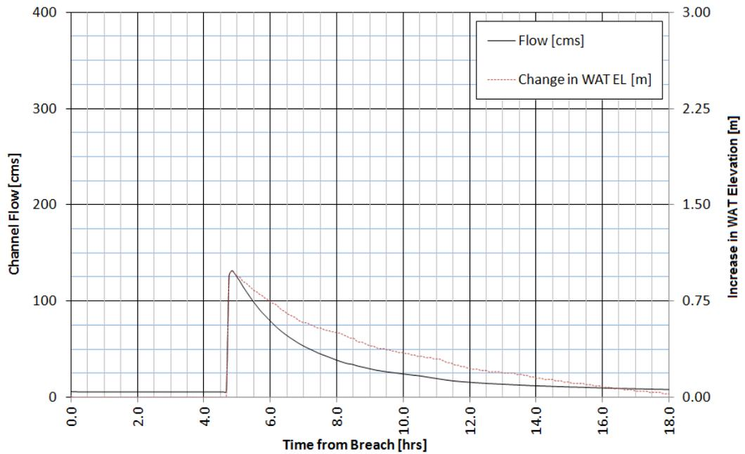
**Figure B.21 - Output for Station 2+311 - 1.0 Hour Dam Breach Duration**
