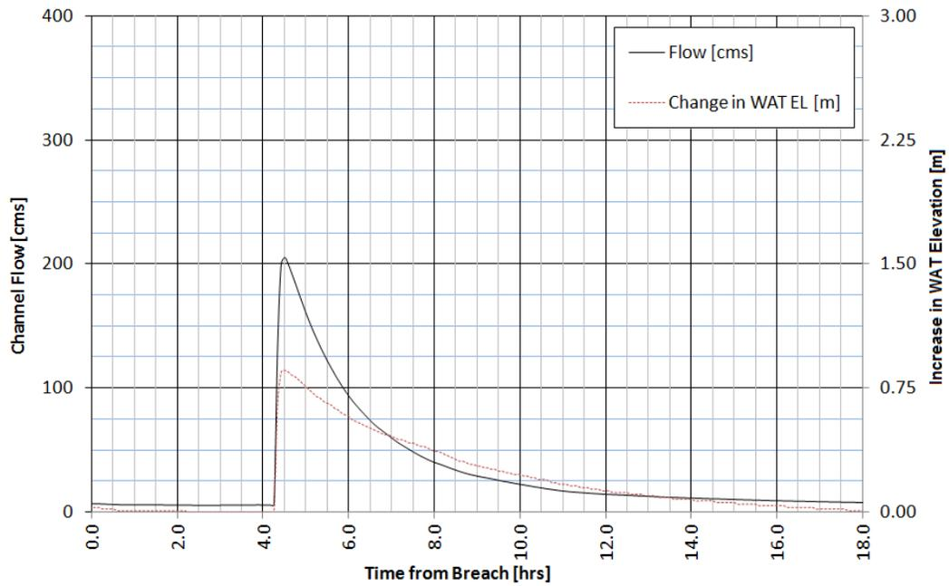
**Figure B.17 - Output for Station 1+792 - 1.0 Hour Dam Breach Duration**
