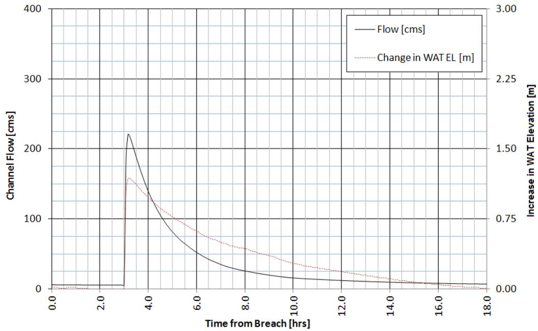
**Figure B.14 - Output for Station 2+987 - 2.5 Hour Dam Breach Duration**
