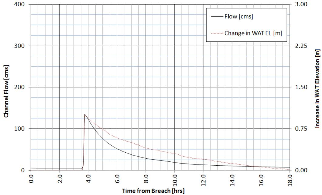
**Figure B.20 - Output for Station 0+247 – 2.5 Hour Dam Breach Duration**
