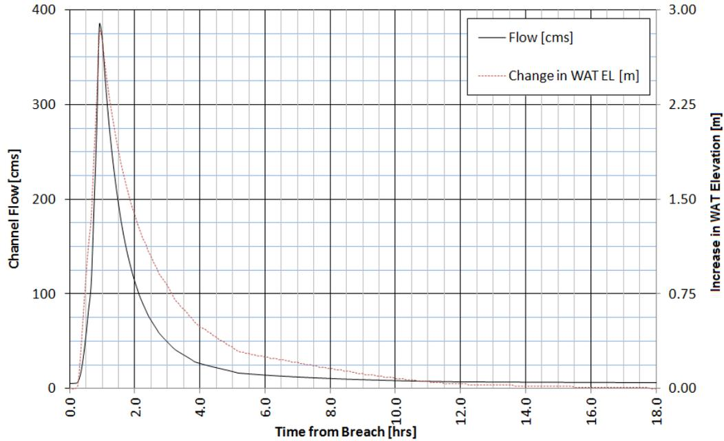
**Figure B.4 - Output for Station 15+376 - 2.5 Hour Dam Breach Duration**
