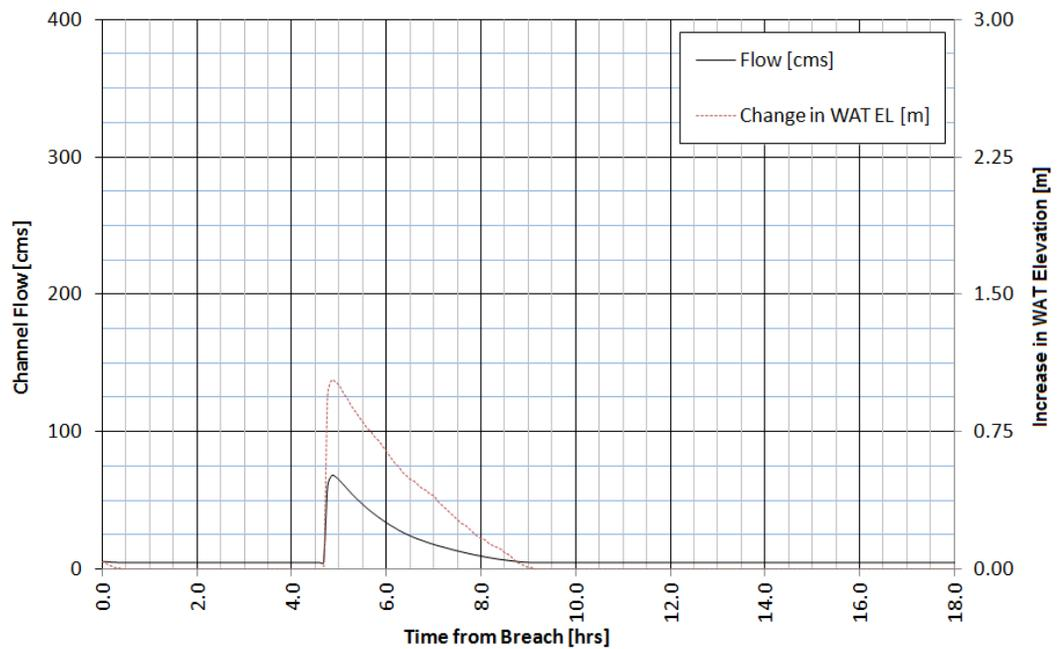
**Figure B.25 - Output for Station 0+161 - 1.0 Hour Dam Breach Duration**
