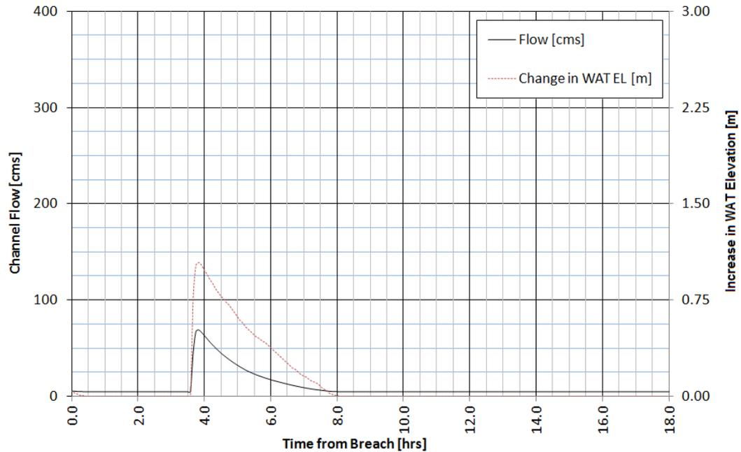
**Figure B.24 - Output for Station 1+461 – 2.5 Hour Dam Breach Duration**
