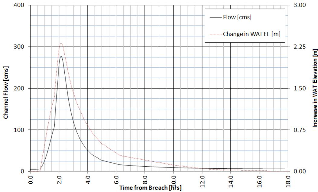
**Figure B.5 - Output for Station 12+076 - 1.0 Hour Dam Breach Duration**
