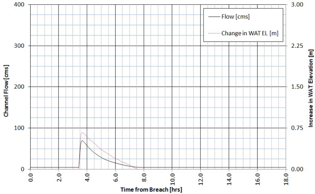
**Figure B.22 - Output for Station 2+311 – 2.5 Hour Dam Breach Duration**
