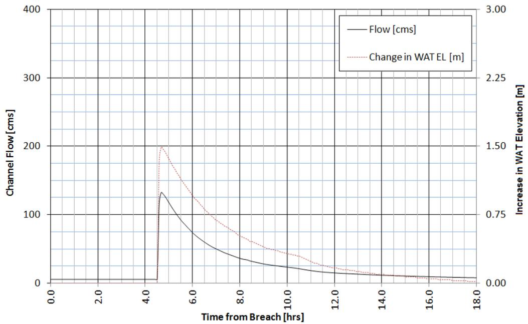
**Figure B.19 - Output for Station 0+247- 1.0 Hour Dam Breach Duration**
