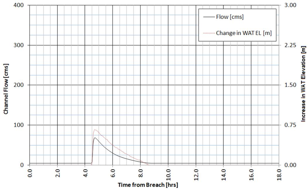
**Figure B.23 - Output for Station 1+461 - 1.0 Hour Dam Breach Duration**
