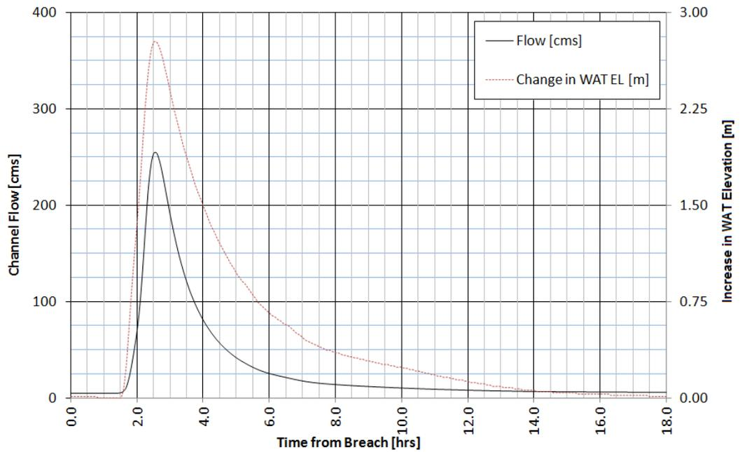
**Figure B.7 - Output for Station 8+976 - 1.0 Hour Dam Breach Duration**
