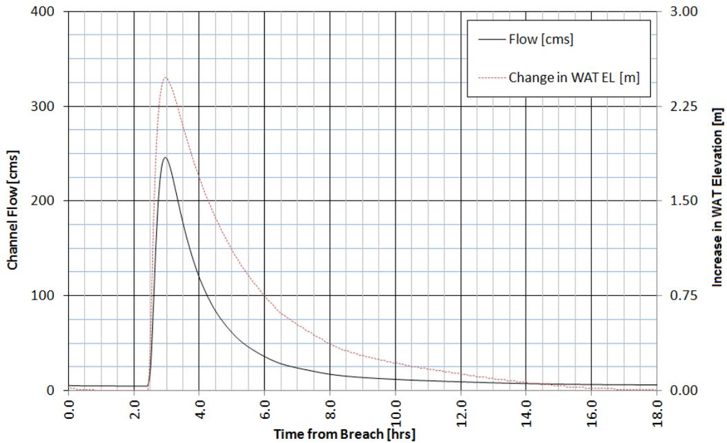
**Figure B.9 - Output for Station 6+026 - 1.0 Hour Dam Breach Duration
