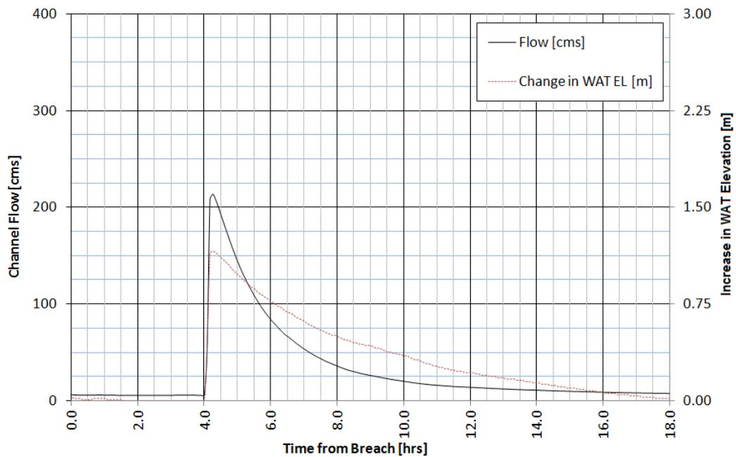
**Figure B.15 - Output for Station 2+431 - 1.0 Hour Dam Breach Duration
