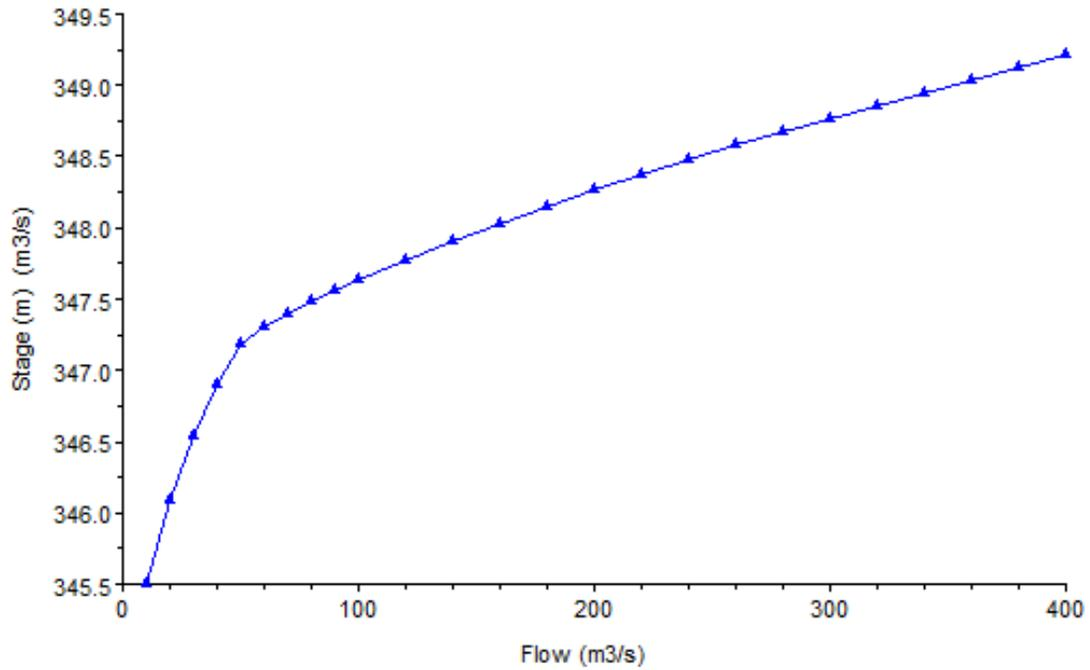
**Figure 3.4 – Breakaway flow to Okanagan Lake: Rating Curve**
