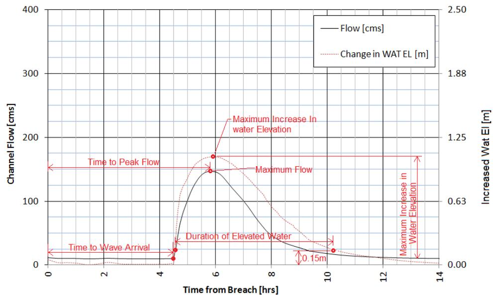
**Figure B.3 - Output for Station 15+376 - 1.0 Hour Dam Breach Duration**
