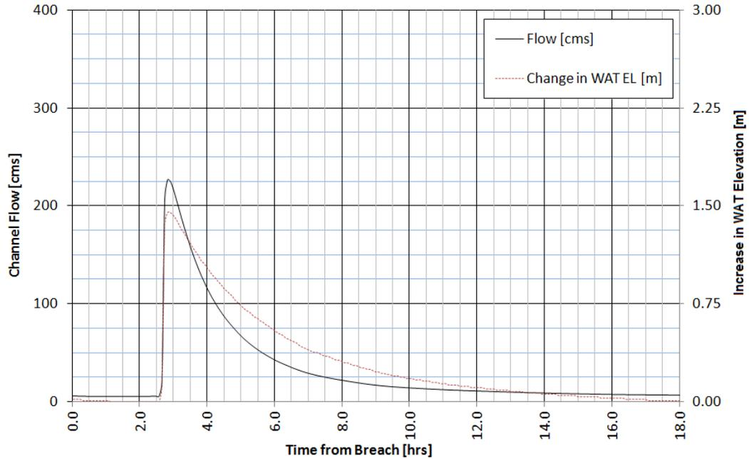
**Figure B.12 - Output for Station 4+226 - 2.5 Hour Dam Breach Duration**
