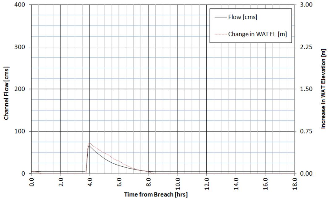
**Figure B.26 - Output for Station 0+161 – 2.5 Hour Dam Breach Duration**
