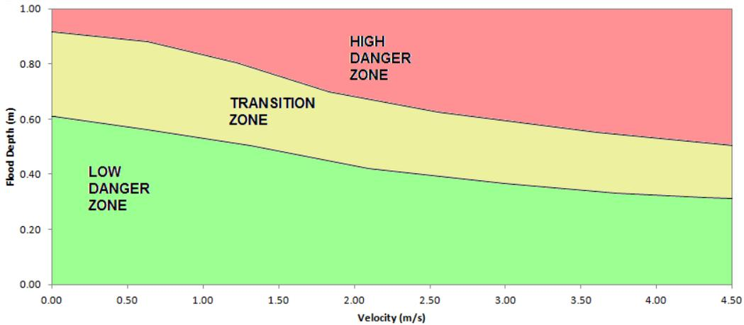
**Figure 4.5 – Estimated Hazard Level for Houses (USBR, 1988)**
