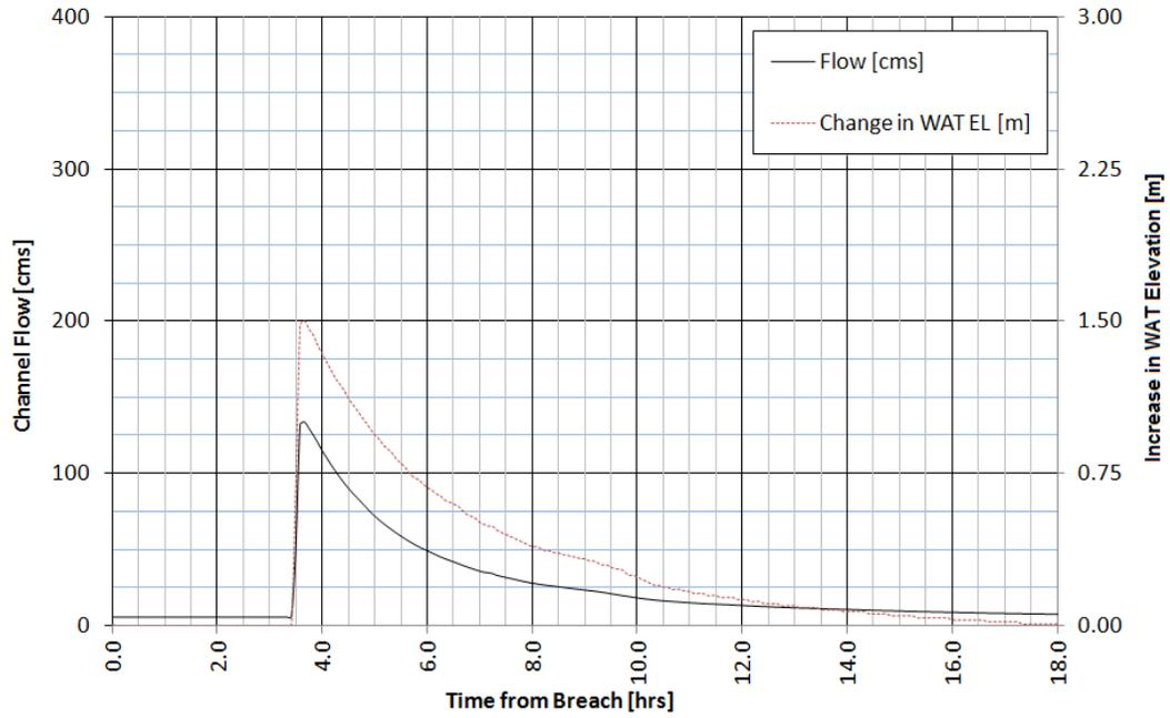
**Figure B.18 - Output for Station 1+792 – 2.5 Hour Dam Breach Duration**
